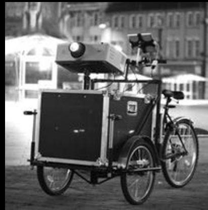
The Light Cycle projection bike, a fully mobile, street art device allowing for travelling projections
